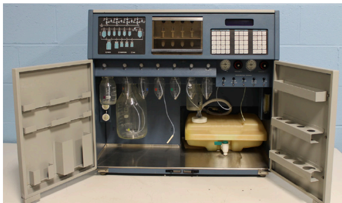
Figure 10.D. A used DNA synthesizer. This equipment is capable of DNA synthesis only (not assembly). It cannot produce continuous nucleic acids longer than 200 bases (0.2 kilobases).
