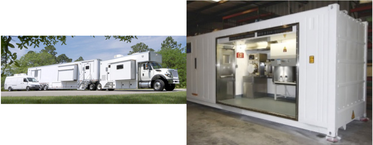
Figure 1.C. Mobile (left) and modular (right) Biosafety Level 3 containment laboratories. The side wall in the right image has been removed for display purposes only.
