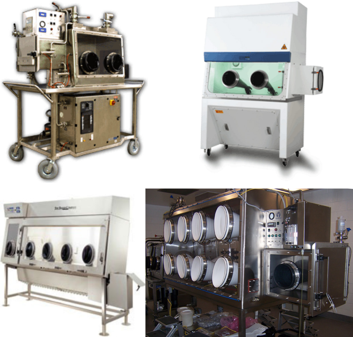
Figure 7.C. Class III biological safety cabinets. Top left: mobile Class III BSC. Top right: Class III BSC with small pass-through box (transfer hatch). Bottom left: multiple-user Class III BSC with dunk tank. Bottom right: extra-large Class III BSC.
