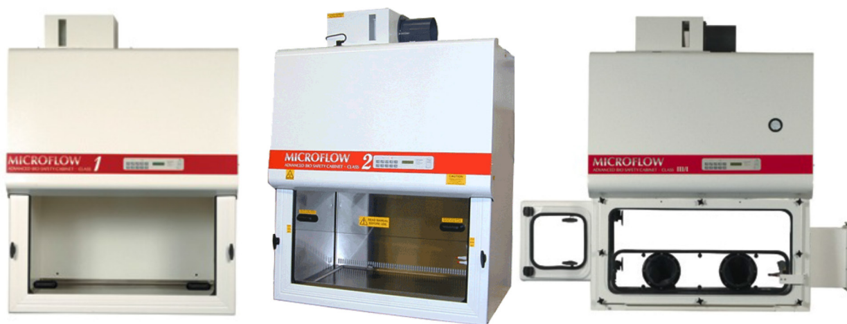
Figure 7.B. Comparison (left to right) of Class I, II, and III biological safety cabinets.
