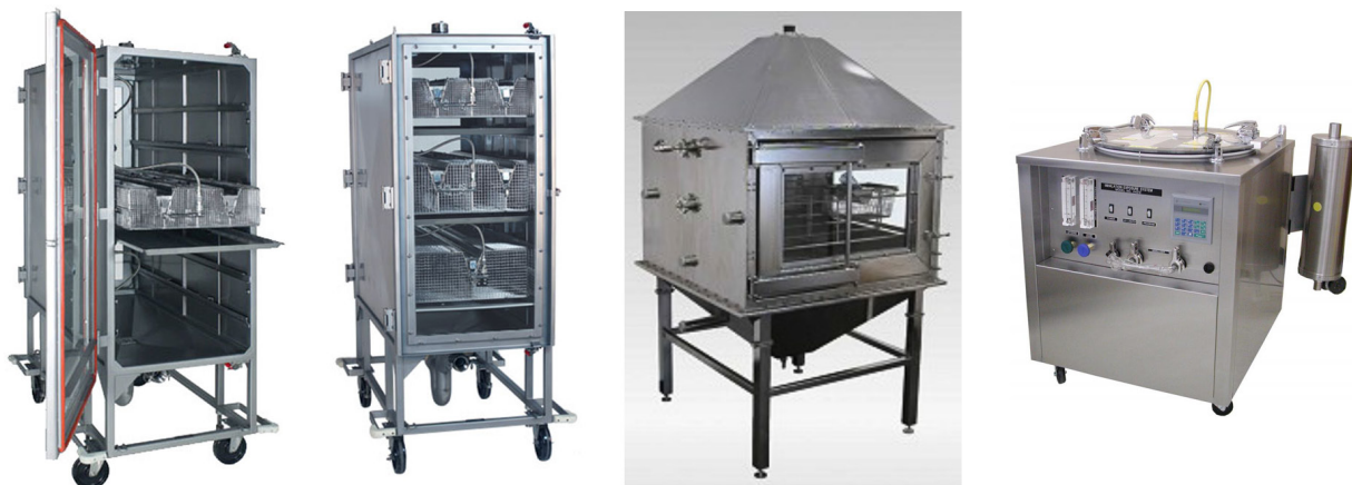
Figure 8.A. Whole-body aerosol inhalation chambers with integral containment systems. Note the connections for sensors and sampling on the side of the chamber in the second photograph from the right. The chamber on the far right contains a basket that can hold multiple mice for whole-body exposure.
