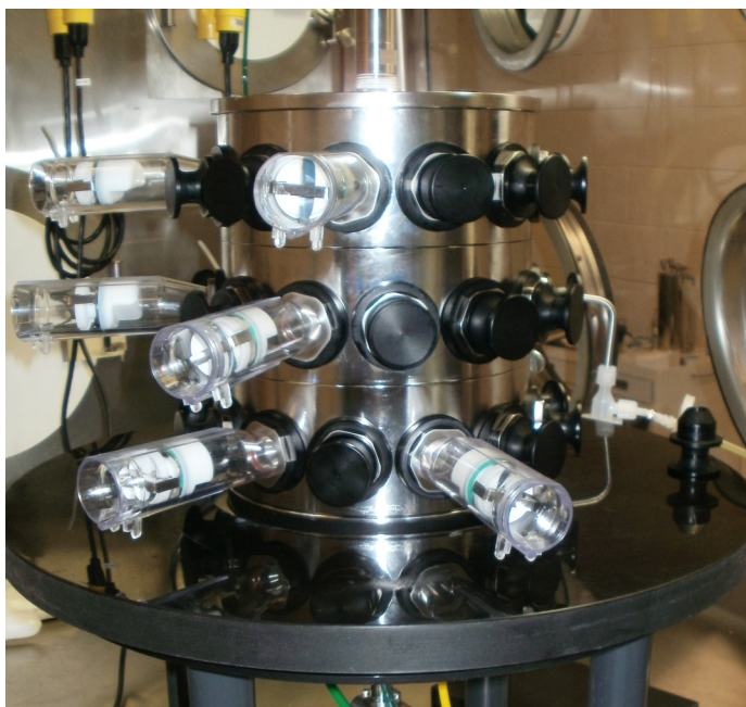
Figure 8.C. Nose-only aerosol inhalation apparatus resident within a Class III Biological Safety Cabinet . Note that the central plenum in the apparatus shown consists of three stackable tiers.
