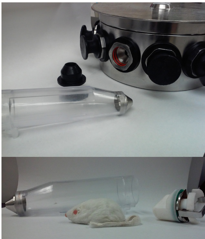
Figure 8.D. Close up views of one tier of a stackable central plenum and closed rodent restraint tubes. Note the polished metal used to construct the plenum as well as the multiple O-ring (orange) seals. A toy mouse is included for size comparison purposes.
