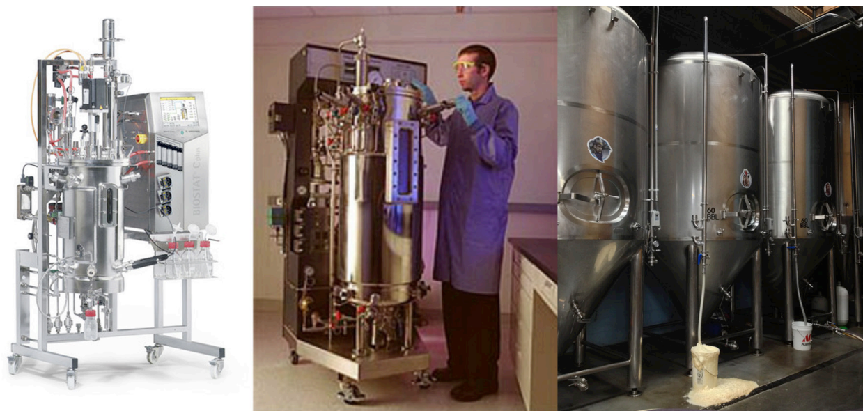
Figure 2.B. Fermenters with different capacities: 15–30 litre laboratory/pilot scale (left); 90-litre pilot scale (centre); 7000 litre production scale (right).
