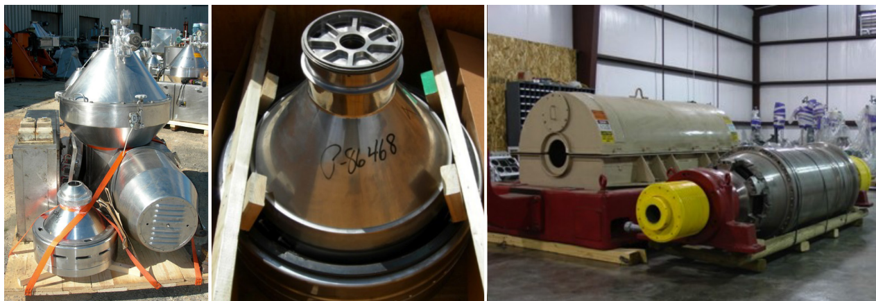
Figure 3.E. Separators, decanters, and their components packaged for shipping.
