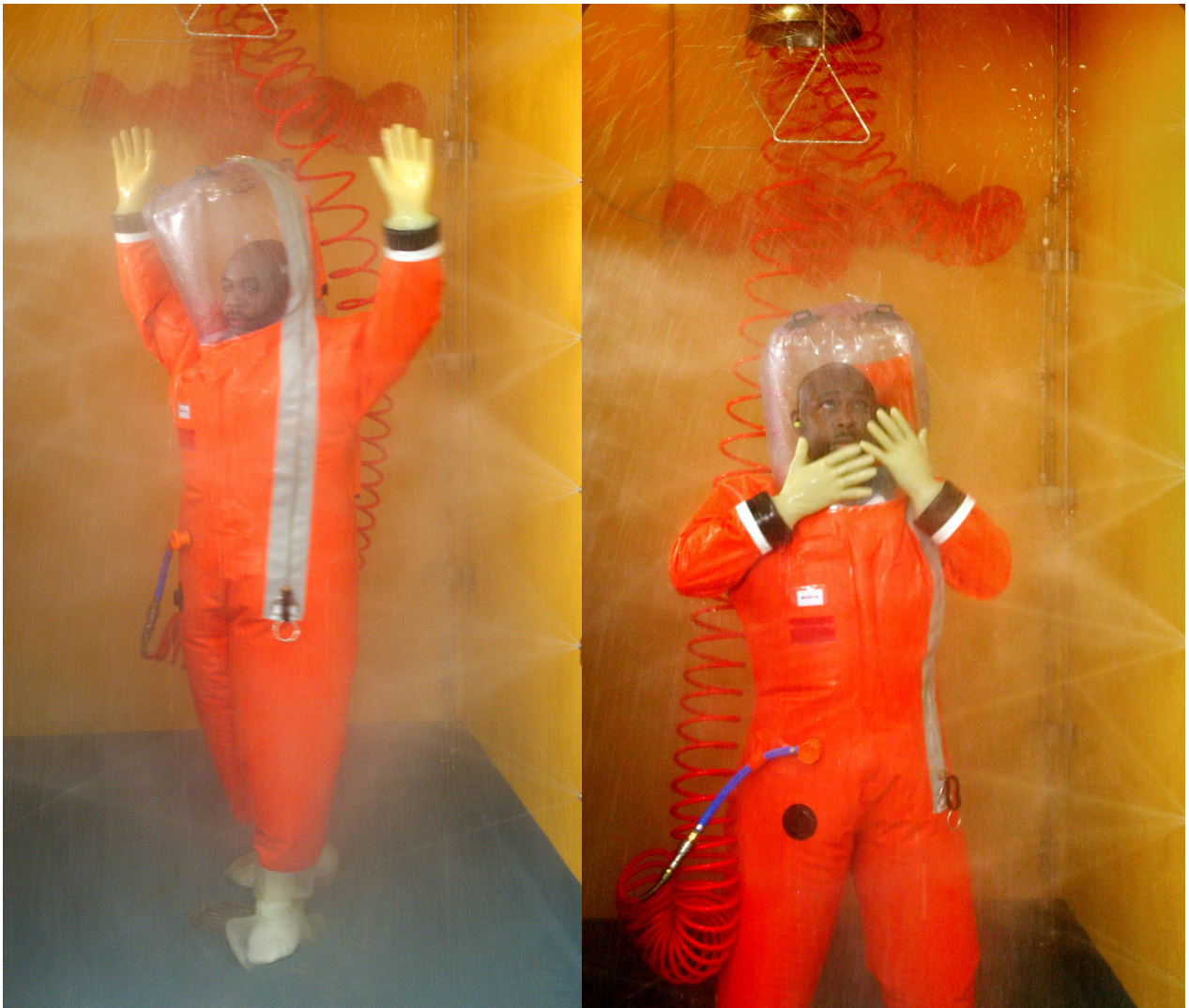
Figure 1.E. Two views of a breathing air suit decontamination shower.
